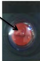
Photo of Pressure adjust valve in open position achieving minimum pressure. This is to show you what the minimum pressure setting will look like for comparison purposes. At this point of the set up process you want the regulator valve closed showing max pressure, as below.
